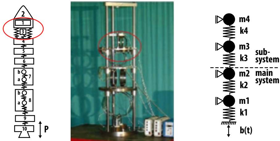
Figure 9.12. Test set-up and model for the real-time substructure tests.
