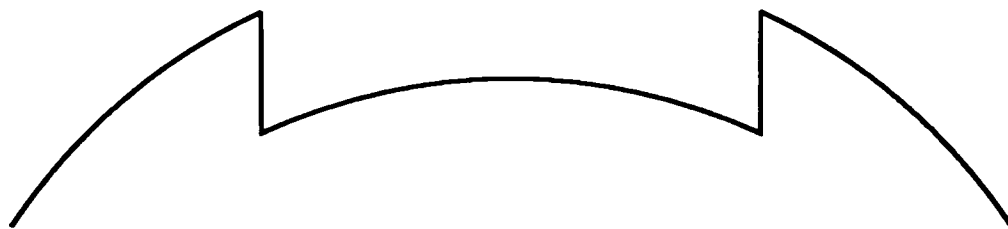
Figure 2.4: Predicted intensity profile of specularly reflecting concave non-Lambertian radiator
