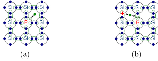
Figure 2.2: Schematics of the silicon lattice in case n-doped (a) and p-doped (b) material.
