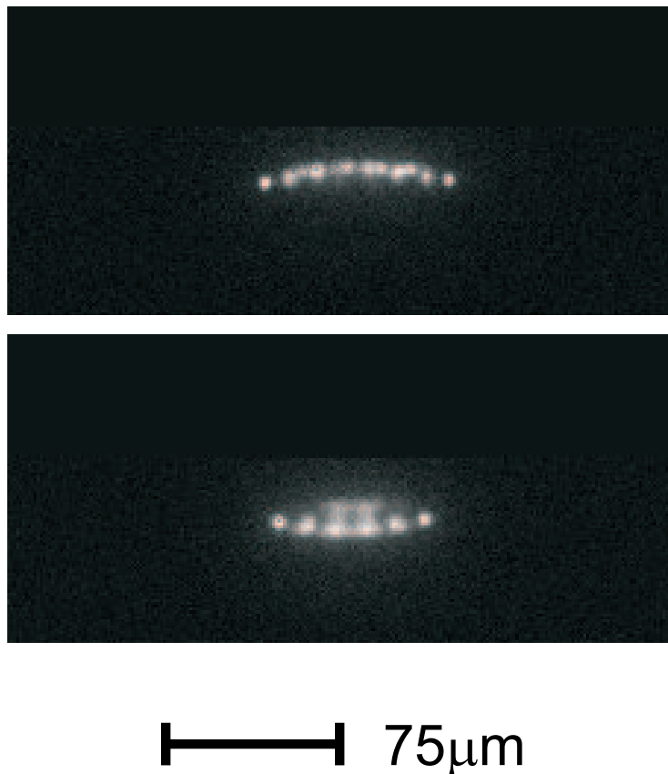
Figure 7.24: Image of a two-species ion crystal. In the upper image we tune the Doppler cooling lasers to the relevant transitions in ^{40}\text{Ca}^+ ; in the lower image these are tuned to the equivalent transitions in ^{44}\text{Ca}^+ . The scale is given above.
