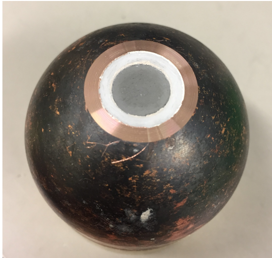
Figure C.1: Porous UHTC sample sealed in the probe head before testing.
