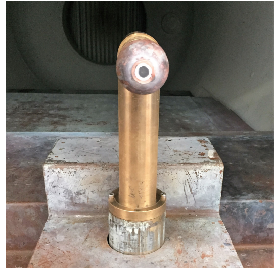
Figure C.2: Probe head mounted in the PWK4 plasma wind tunnel.
