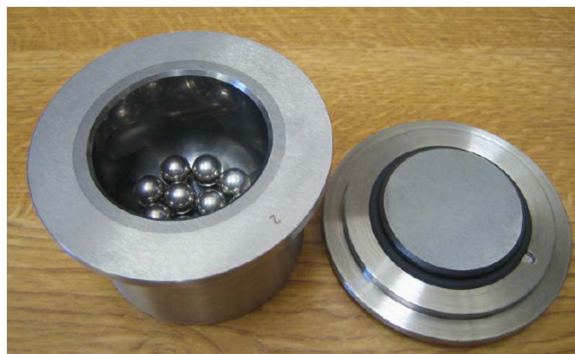
Figure 2.1.4: Mechanochemical mill vessel and balls
