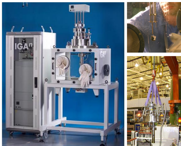
Figure 2.8.1: Left: The entire IGA n unit. Upper right: Inside the reaction vessel, showing the balance and sample bucket. Lower right: A loaded sample being craned into a diffractometer.
