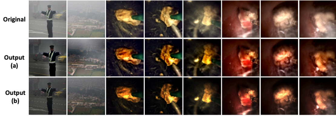
Figure 6.3: Dehazing results using approach (a) presented in [242] and approach (b) presented in [243] implemented on two natural scene images followed by three in vitro and three animal dataset ureteroscopy images
