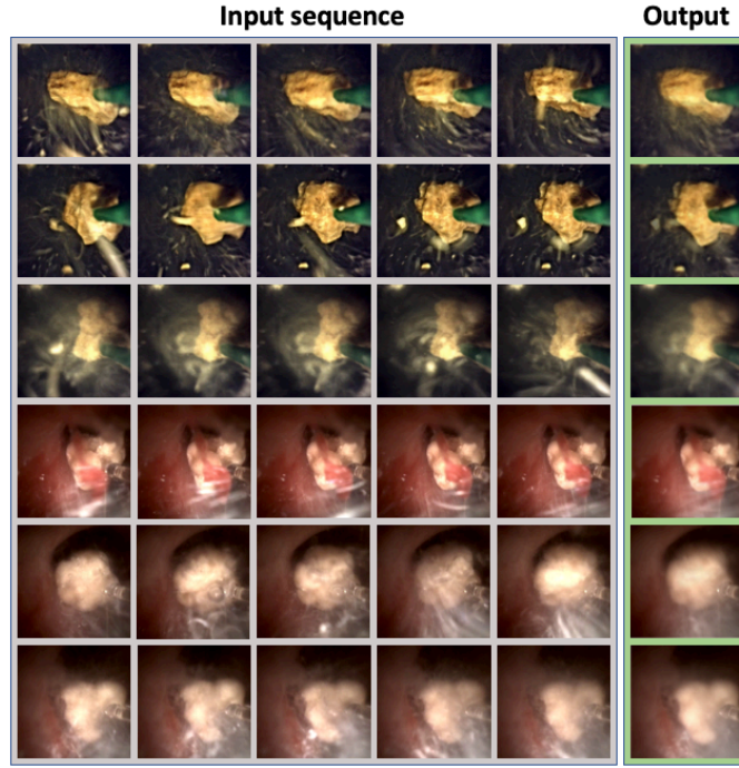
Figure 6.2: Results for temporal averaging of pixel intensities (across five adjacent frames) shown for three in vitro and three animal dataset samples
