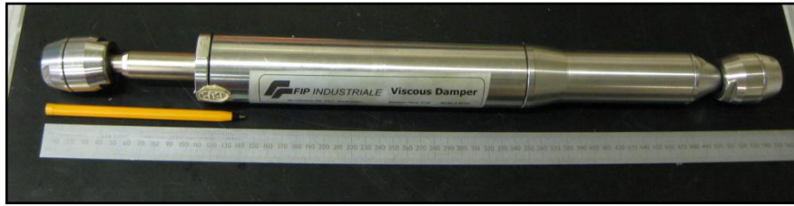
Figure 4.4. Acquired Fluid Viscous Device
