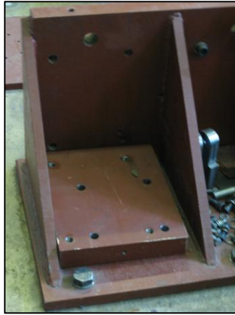
Figure 4.7. Permanent Anchor and Adapter Plate
