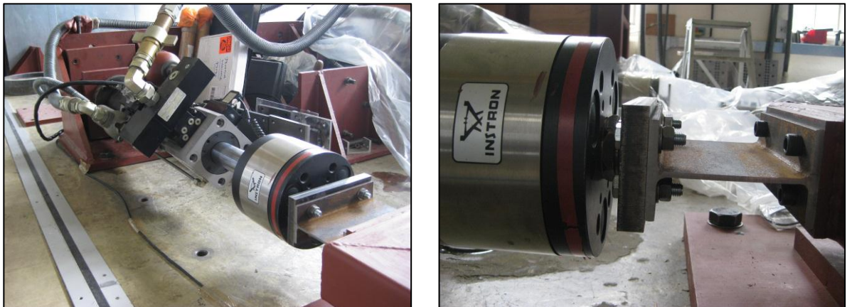
Figure 4.8. Actuator Mounting (Left) and Hinge (Right)
