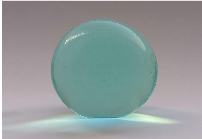
Figure 3.1: A hydrogel bead rests on a rigid planar substrate. Water may be expelled from the bead as it deforms, forming a liquid bridge around the contact that can adhere the bead to the substrate. (The bead depicted has a diameter of approximately 3 cm.)
