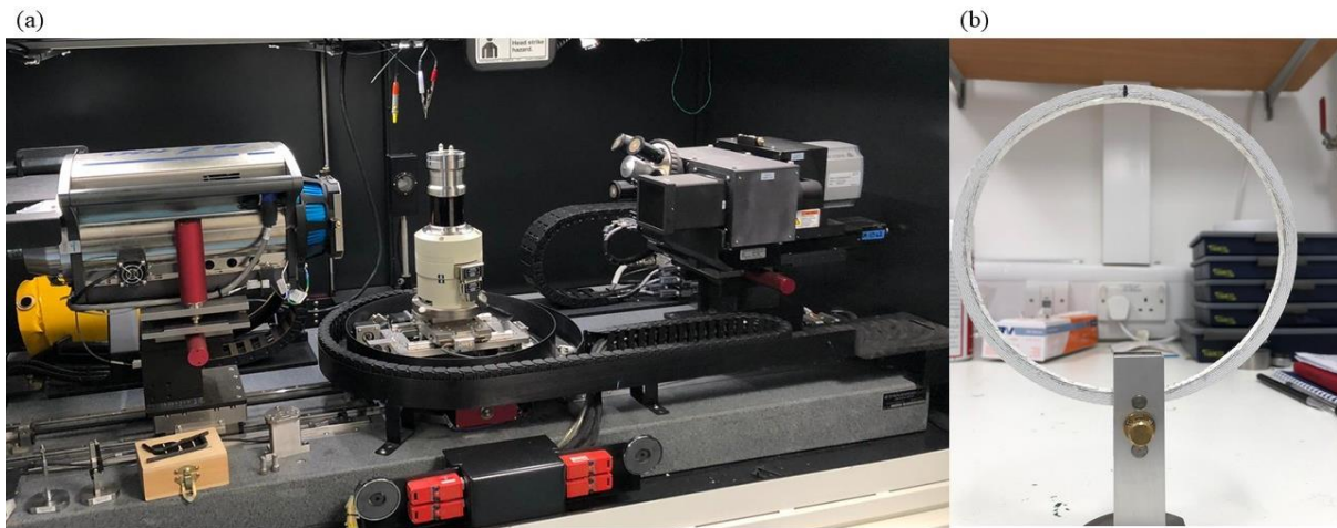
Figure 60: (a) Zeiss Xradia 510 Versa 3D X-ray tomography microscope used to carry out lab based \mu CT analysis (b) a ring sample loaded in a \mu CT holder.
