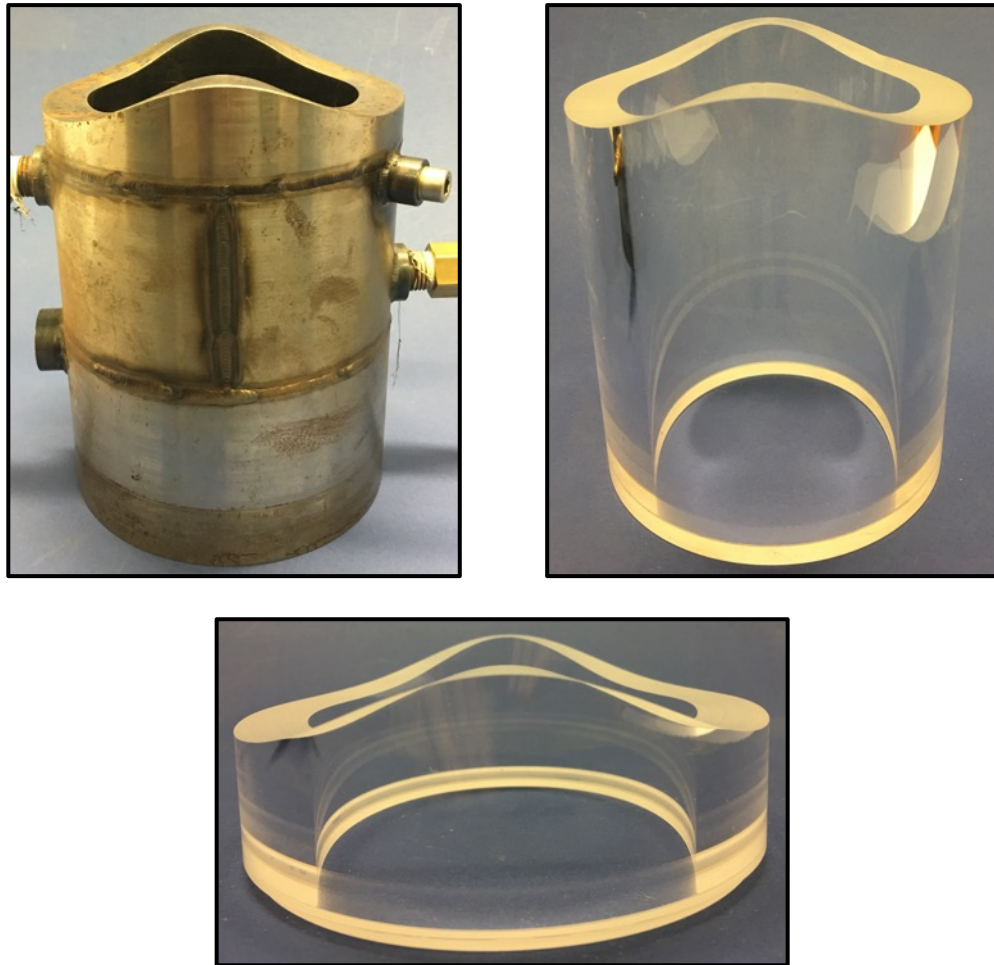
Figure 2.4 Photographs of the cylinder liners available for use in engine: Full steel (top left), full quartz (top right), and quartz annulus (bottom).
