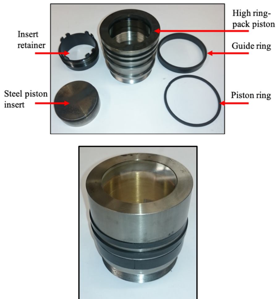
Figure 2.5 An exploded view of the high ring-pack piston and associated components (top), and an image of the low ring-pack piston with transparent quartz piston insert (bottom).
