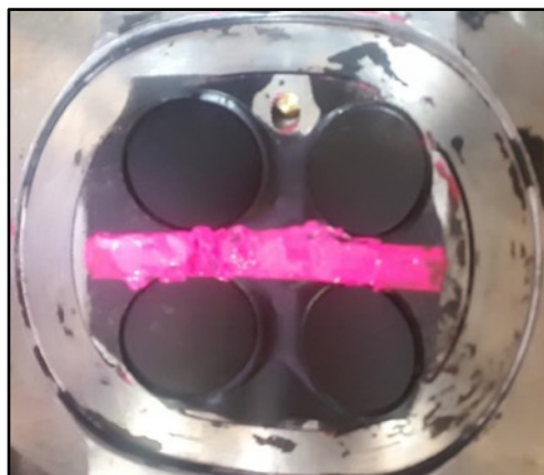
Figure 3.25 A photograph of the cylinder head painted with matt black paint and a strip of fluorescent pink for scatter minimisation (inlet valves are on the right of the image).
