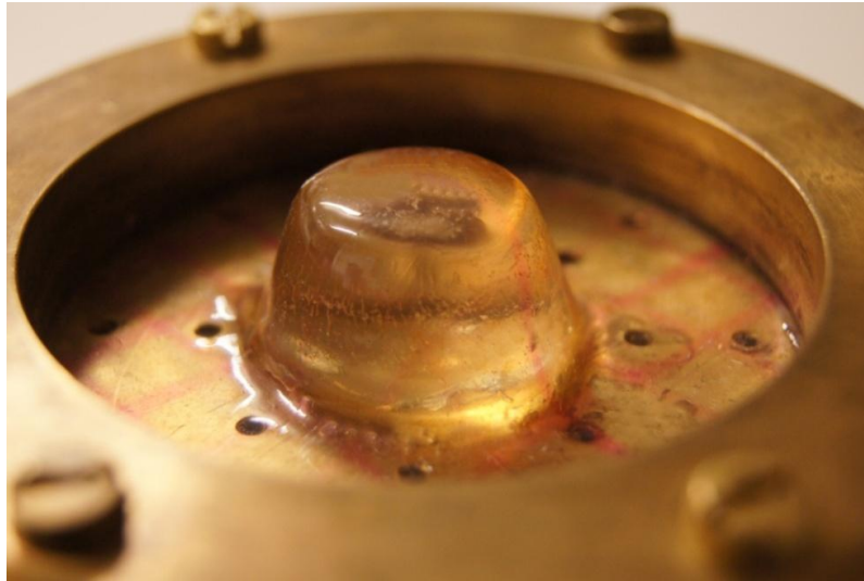
Figure 4.21: Image of swollen hydrogel expander under polyurethane skin.
