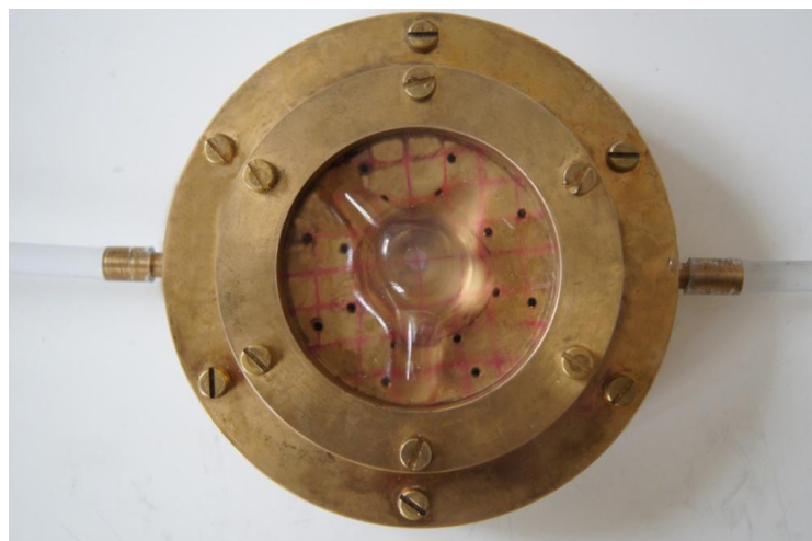
Figure 4.16: Isotropic swelling gel after 24 hrs of hydration under apparatus.
