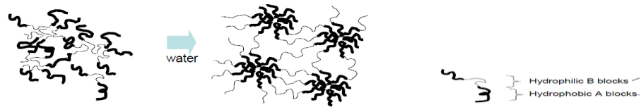
Figure 2.04: Schematic of hydrogel chains showing relaxation of hydrophilic regions when in contact with water. Ref. [13]
