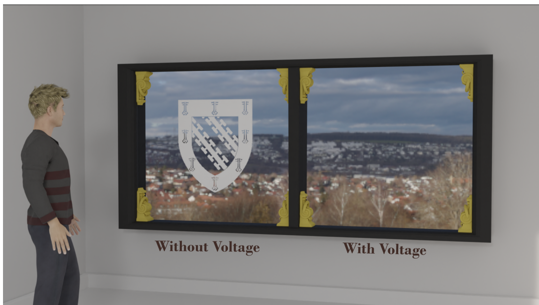
Figure 5.20: Graphical representation of the printed PDLC smart glass concept in which a company logo or emblem can be made to disappear with the application of an electric field.
