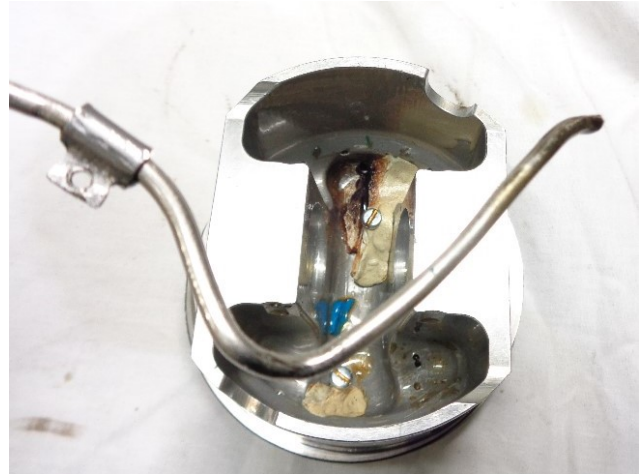
(b) Broken stainless steel sample tube
