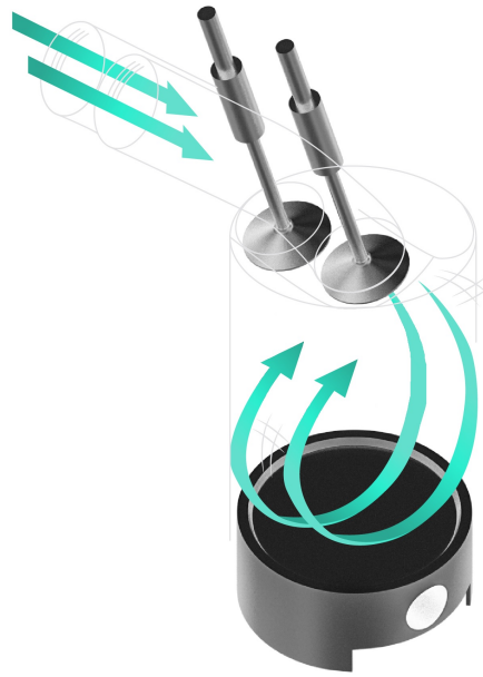
Figure 2.1: In-cylinder ‘tumble’ bulk motion, adapted from [23]
