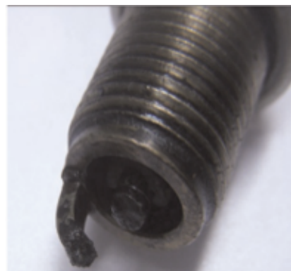
(b) Spark plug damage
