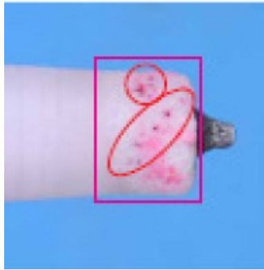
Figure 2.10: Insulator with dielectric puncture. Images courtesy of Jaguar Land Rover.
