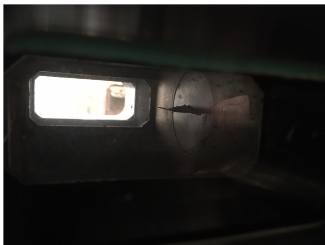
(b) Knife blade – installed position in the end wall of the CDST
