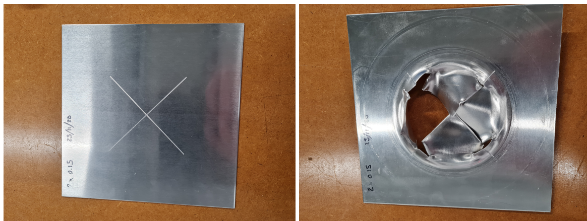
(a) New diaphragm, 2 x 0.15mm crossing scores
