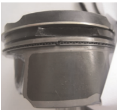
(a) Piston damage
