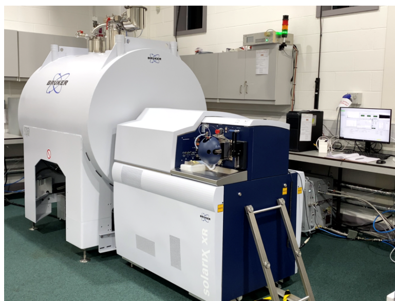
Figure 5.20: Bruker 15 T Fourier Transform Ion Cyclotron Resonance Mass Spectrometry (FTICR MS), housed at the University of Warwick.
