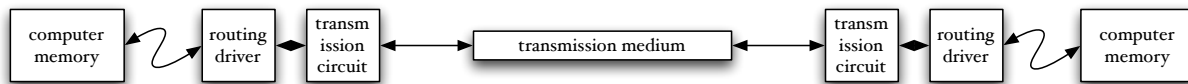
Figure 6.3: Schematic showing the interconnect sequence in a single bidirectional interconnection line. The energy consumption model treats each of these stages as a separate component.
