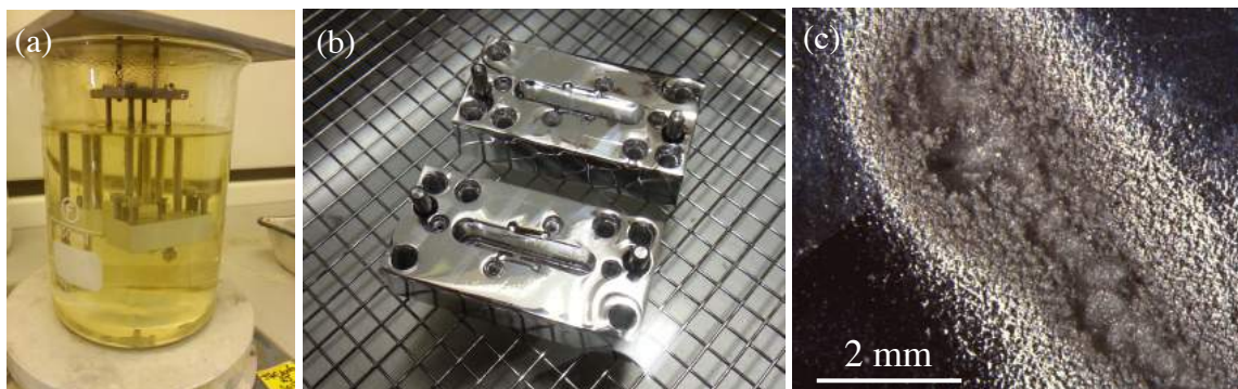
Figure 5.5: (a) A picture of the aluminium etching setup. (b) The smooth, but uneven, etched surfaces of a 5N5 pure aluminium cavity. (c) Example of spots where the acid was not properly neutralised and continued the etching.
