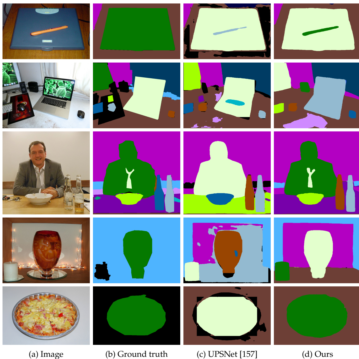
Figure 5.11: Qualitative results on the COCO dataset. Column (c) is produced by running the publicly available inference script of [157]. With our parametrised panoptic segmentation submodule, we are able to produce more coherent, accurate, and visually appealing predictions than the parameter-free approach of [157].
