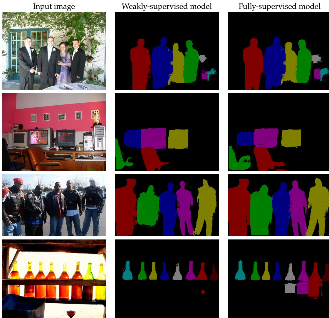
Figure 4.9: continued . The first and second rows show examples where the results of the two models are similar. In the third row, the weakly-supervised model does not segment the “green person” as well as the fully-supervised model. In the last row, both weakly- and fully-supervised models have made an error in not completely segmenting each of the bottles.
