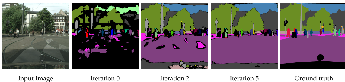
Figure 4.4: By using the output of the trained network, the initial approximate ground truth produced according to Sec. 4.3.2 and 4.3.3 (Iteration 0) can be improved. Black regions are “ignore” labels over which the loss is not computed in training. Note for instance segmentation, permutations of instance labels of the same class are equivalent.
