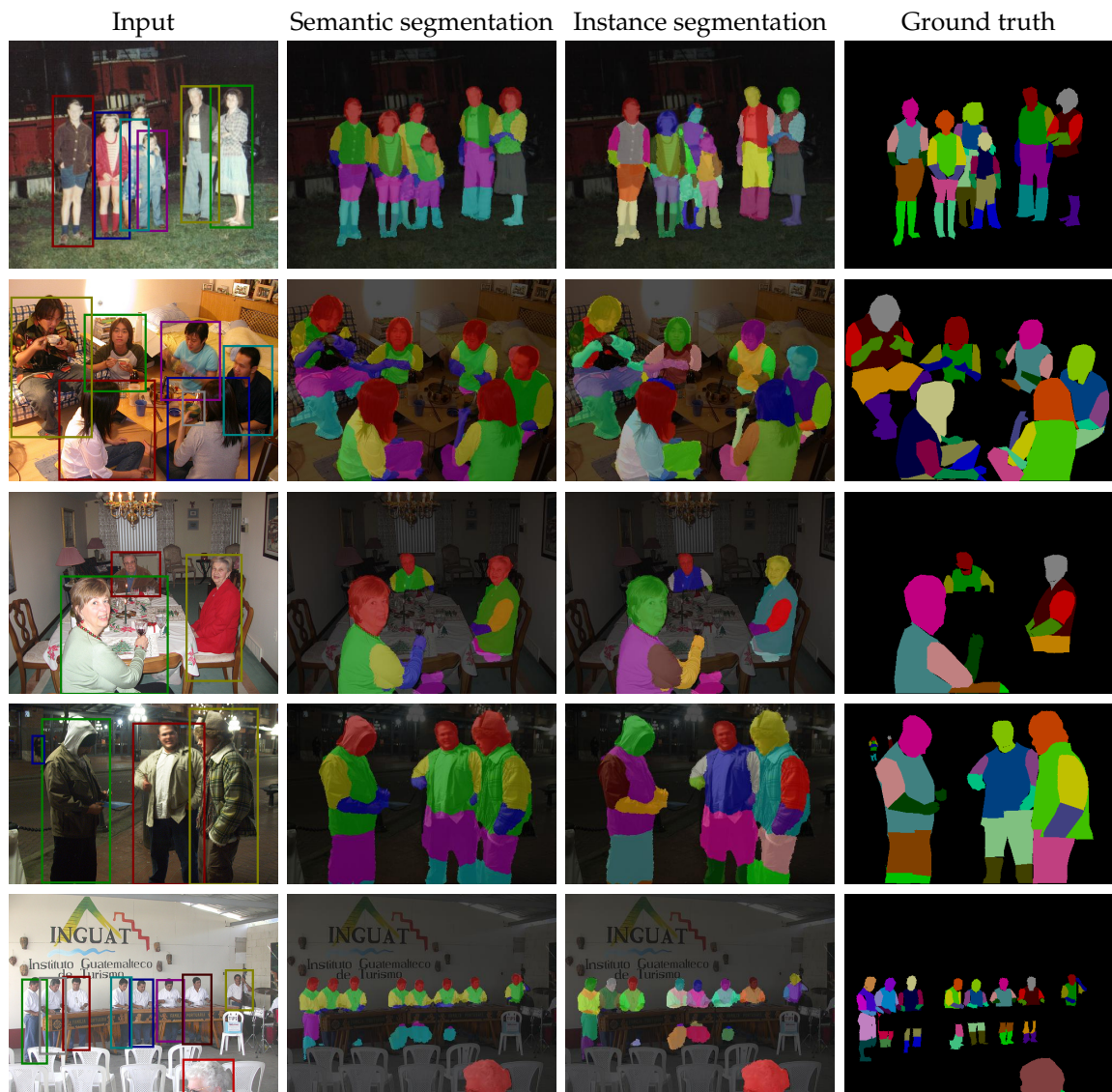
Figure 3.4: Some results of our system. The first column shows the input image and the input detections we obtained from training the R-FCN detector [32]. The second and third columns show our final semantic segmentation (Sec. 3.3.4) and instance-level part segmentation. First row : our network can deal with poor bounding box localisation, as it manages to segment the third person from the left although the bounding box only partially covers her. Second row : our method is robust against false positive detections because of the box term. Observe that the bowl of the rightmost person in the bottom row is falsely detected as a person, but rejected in the final prediction. Following rows : we are able to handle overlapping bounding boxes by reasoning globally using the Instance CRF.
