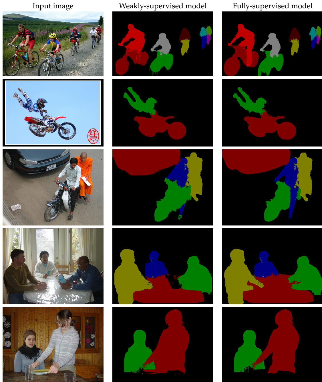
Figure 4.9: Comparison of our weakly- and fully-supervised instance segmentation models on the Pascal VOC validation set. The weakly-supervised model typically obtains results similar to its state-of-the-art, fully-supervised counterpart. However, the fully-supervised model produces more accurate and precise segmentations, as seen in the last two rows.
