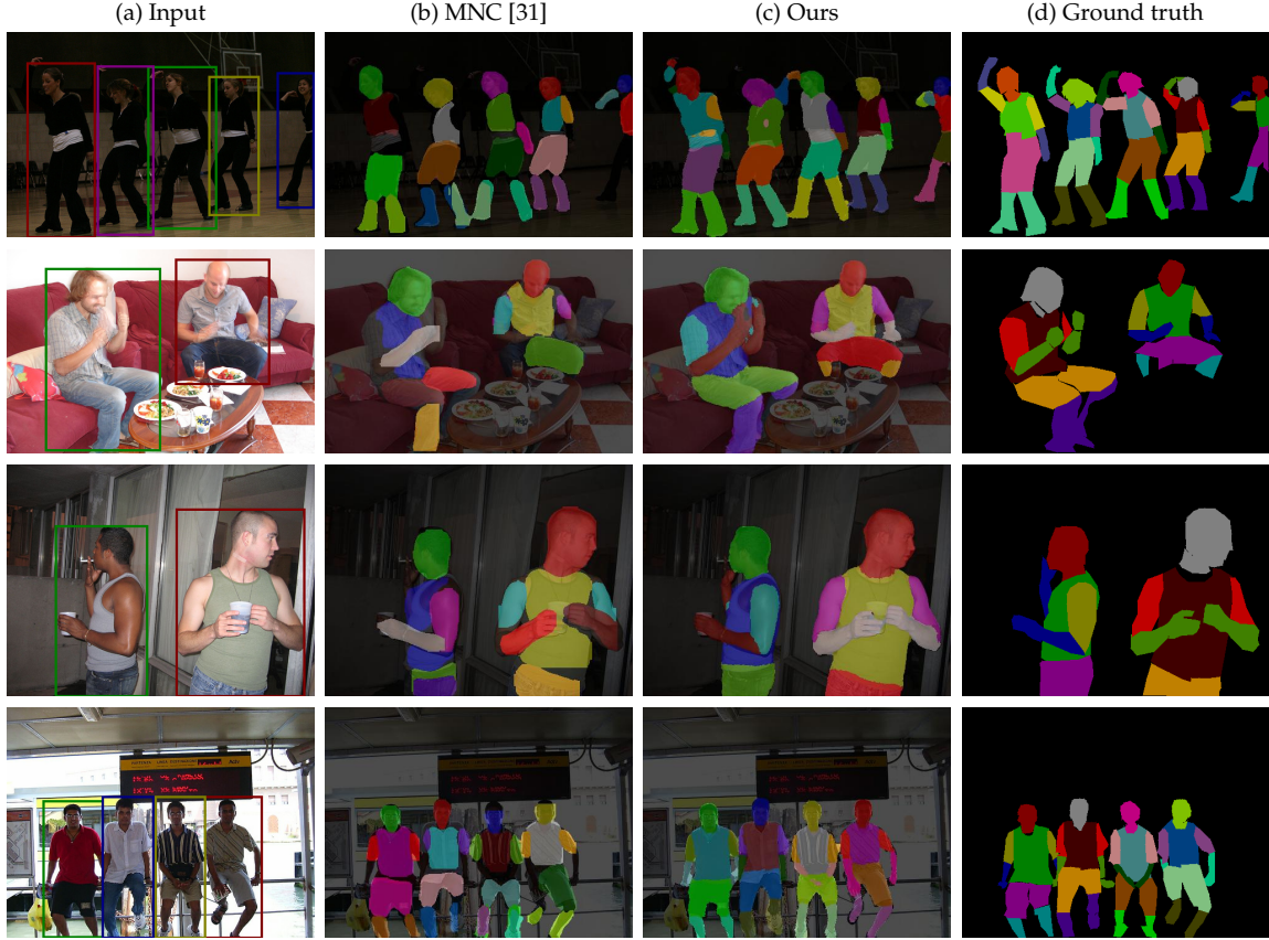
Figure 3.8: Comparison to MNC on the Pascal Person-Parts [24] test set. First row : unlike MNC which predicts for each part instance independently, our method reasons globally and jointly. As a result, MNC predicts two instances of lower legs for the same lower leg of the second and third person from the left. Furthermore, with a dedicated category-level segmentation module, we are less prone to false negatives, whereas MNC misses the legs of the rightmost person, and the lower arm of the second person from the right. Second row : while we can handle poor bounding box localisation because of our global potential term, MNC is unable to segment regions outside the bounding boxes it generates. Consequently, only one lower arm of the person on the left is segmented as the other one is outside the bounding box. The square corners of the segmented lower arm correspond to the limits imposed by the bounding box which MNC internally uses. Third row : By analysing an image globally and employing a differentiable CRF, our method can produce more precise boundaries. As MNC does not perform category-level segmentation over the entire image, it has no incentive to produce a coherent and continuous prediction. Visually, this is reflected in the gaps of “background” between body parts of the same person. Fourth row : MNC predicts two instances of the lower leg for the second person from the right, and fails to segment any lower arms for all four people due to the aforementioned problems.
