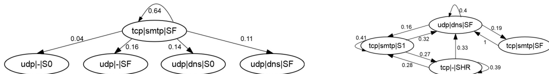
Figure 9.12: Markov Chain for Sality ( right ) and Geodo ( left ) spam behavior (only state transition probabilities, where p > 0.1 ).
