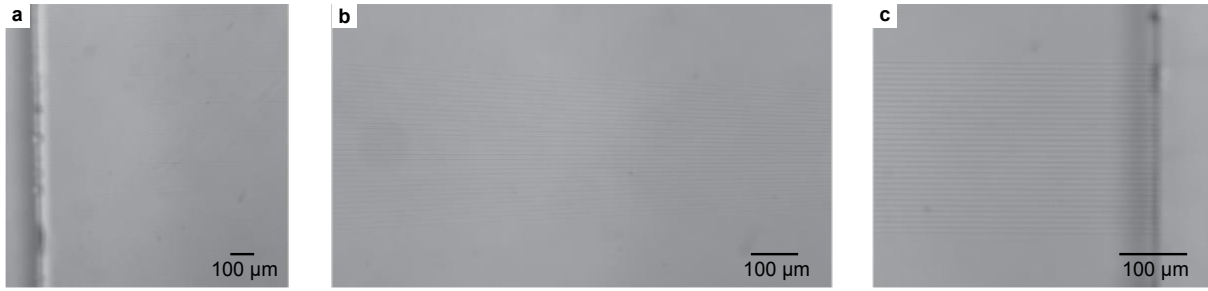
Figure S5 Top view microscopic images of a 32-channel photonic chip. The 32-channel chip was measured to have similar performance in terms of cross-coupling and losses to the 8-channel chip described in main text. a Image at the chip input, where the channel are spaced by 127\ \mu\text{m} to match the VGA. b Image at the middle part of the chip where the channel spacing is reduced. c Image at the chip output, where the channel spacing is reduced to 8\ \mu\text{m} .
