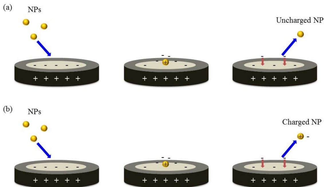
Figure 2.3: Two types of capacitive impacts. The electrode double layer is perturbed and restored by an impacting particle. Either (a) an uncharged or (b) a charged particle is formed after the collision.
