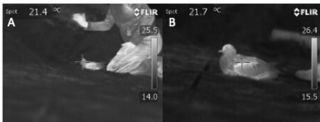
Figure S2.1. Two photos showing a bird 4m ( A ) and 2m ( B ) away from the camera. The Motion-Based Multiple Object Tracking module in MATLAB (R2017a) recognised moving objects bigger than 20 pixels and smaller than 4000 pixels. The approximate calculations revealed that it would mean that birds were minimum 5m away and maximum 85m away from the camera.
