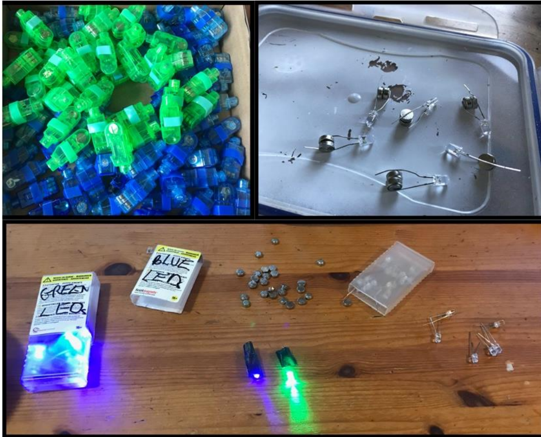
Figure S3.1. LEDs used for the experiment in their casing (top left) and after the casing were taken off (top right). Bottom picture shows a box of ready for experiment LED lights, batteries and LEDs ready to be assembled. There are two lights in the middle: one in a full hoodie made of tesa tape (blue), and one without a hoodie (green).
