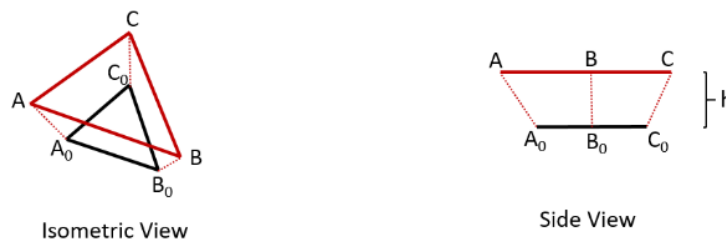
Figure 2.10: Tet Prism Surface Redefinition for ICI Accretion Extrusion taken from Porter et al. [110].
