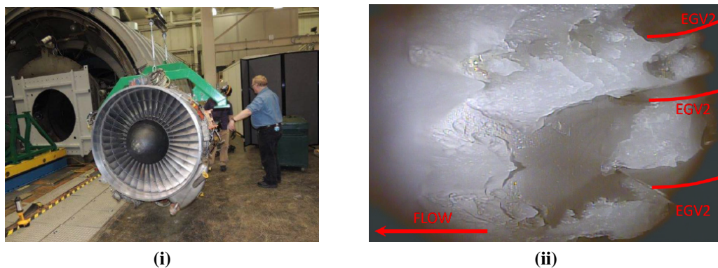
Figure B.3: (i) Lycoming ALF502 - R5 LF01 Flight Test Engine used to recreate ICI conditions causing un-commanded rollback [104]. (ii) Ice Crystal Icing observed on the outer shroud downstream of the ALF502 EGV's [49].
