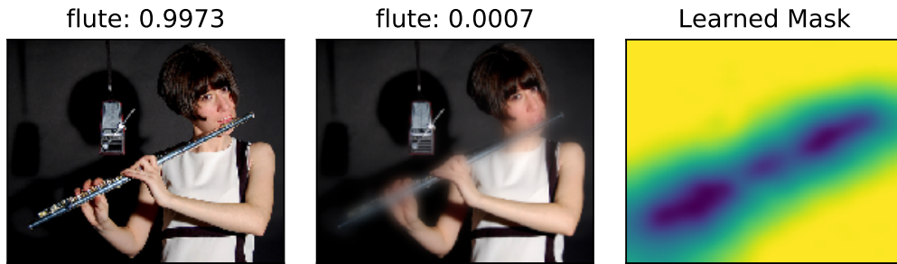
Figure 1.2: Meaningful perturbations (Fong et al., 2017). In this example, a mask is learned (right) and used to edit ( i.e. blur) an image (middle) so that the image classifier’s “flute” prediction is changed from 99% confidence to less than 1% confidence (left: original image).
