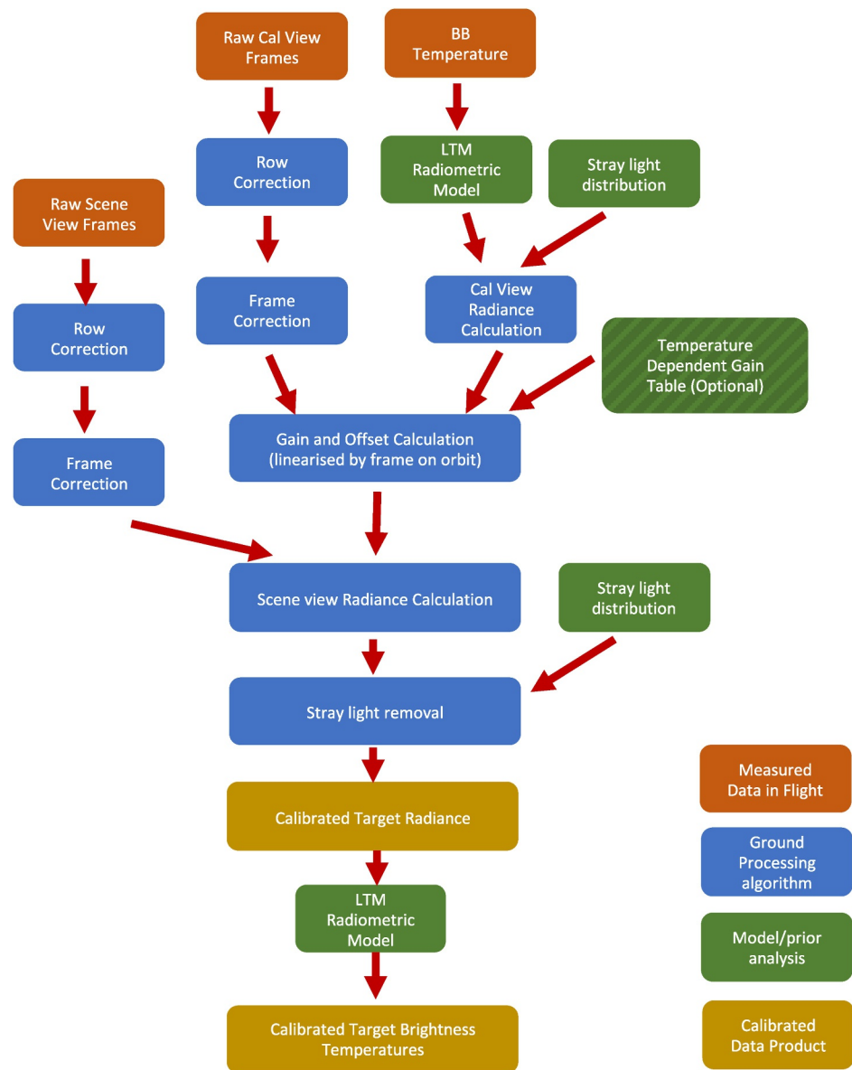
Figure 14. Calibration pipeline used to generate the level 1 and higher products for the Planetary Data System (PDS).
