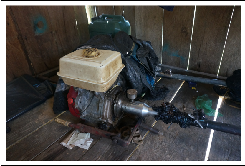
Figure 2. A typical peke-peke boat's motor, whose tail extends another metre to the right. The sole of a rubber boot serves to replace the original lid of the tank. Photograph by author.
