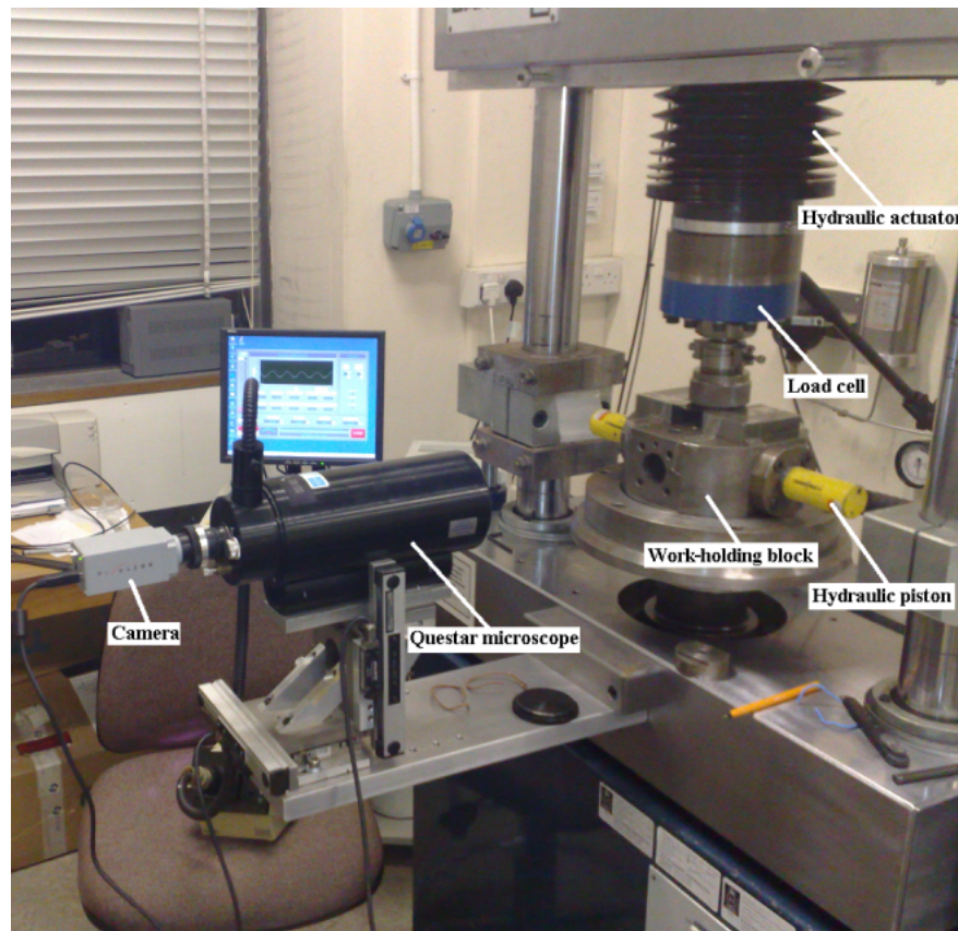
Figure 6.11: Photograph of the Dartec servo-hydraulic tensile testing machine showing various features of the test setup including the camera and Questar microscope used for obtaining digital images.
