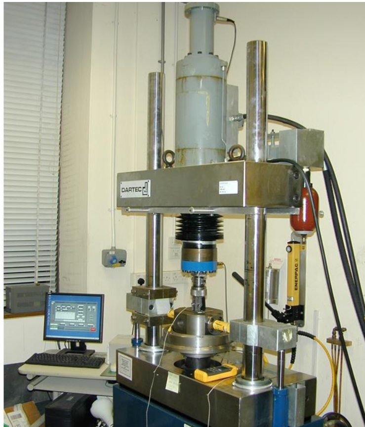
Figure 3.11: Photograph showing the Dartec servo-hydraulic tensile testing machine with the test fixtures attached.
