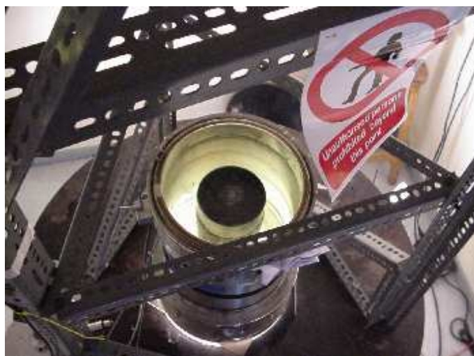
Figure 2.2: Close-up view into the annular tank from above.
