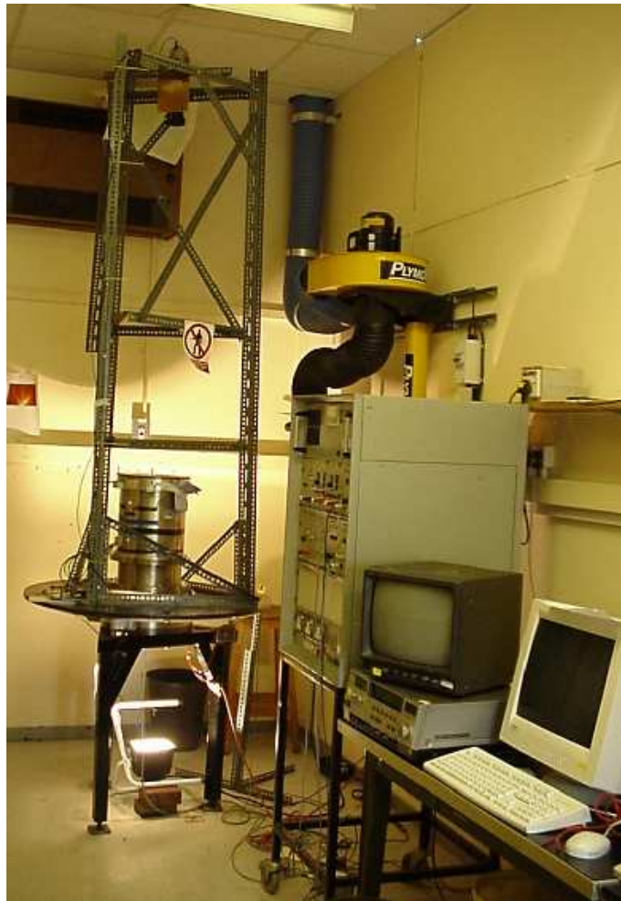
Figure 2.1: The two-layer annulus apparatus and control equipment. From left to right: the rotating turntable, mounted with the annulus and with a tall metal frame to support the video camera; an amplifier which powers the turntable rotation and lid rotation; a television and video recorder to watch and record live images from the camera; and a computer with a frame-grabber installed to digitize and save selected images.
