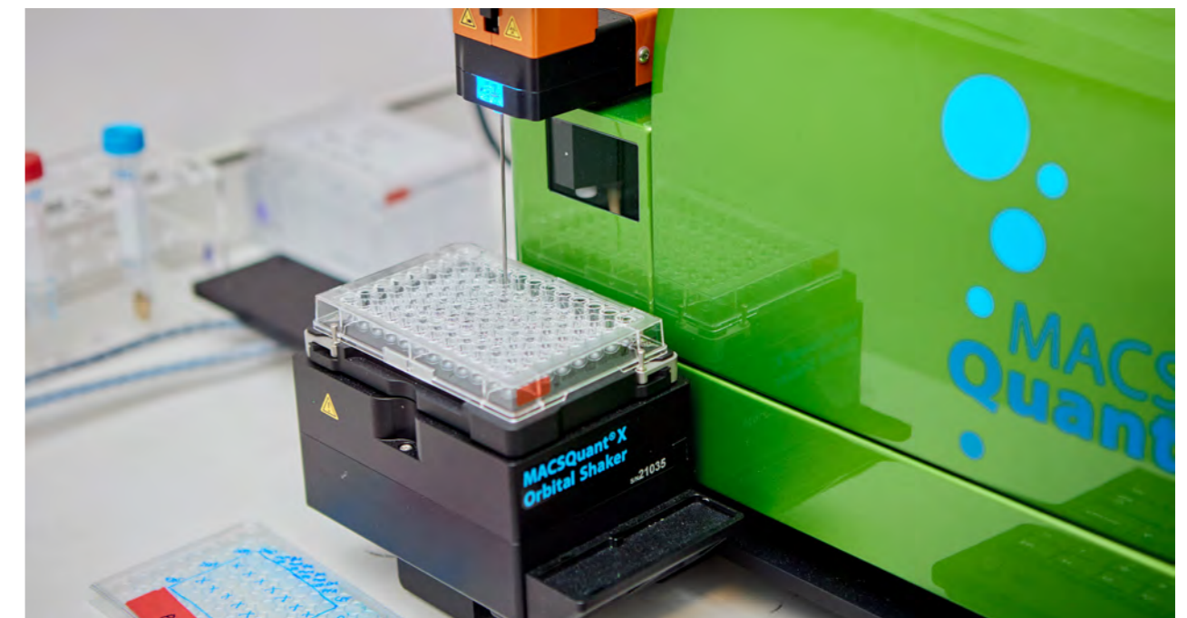
A compact flow cytometer made to provide maximum speed and reliability in high-throughput screening used in Susanna Dunachie's Oxford lab. © MORU 2022. Photographer: Samuel Allard.
