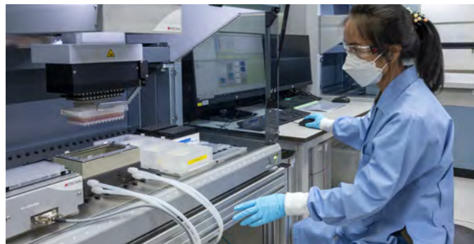
Sample processing and extraction using an automated liquid handler. © MORU 2022. Photographer: Gerhard Jøren.
