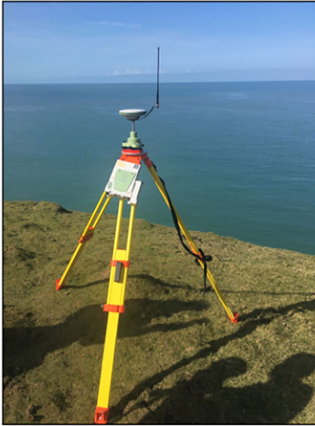
Figure 2. The RTK unit used by the RCAHMW pictured here at Castell Bach, an iron-age promontory fort in Ceredigion, Wales. Photo by Sterling Mackinnon.
