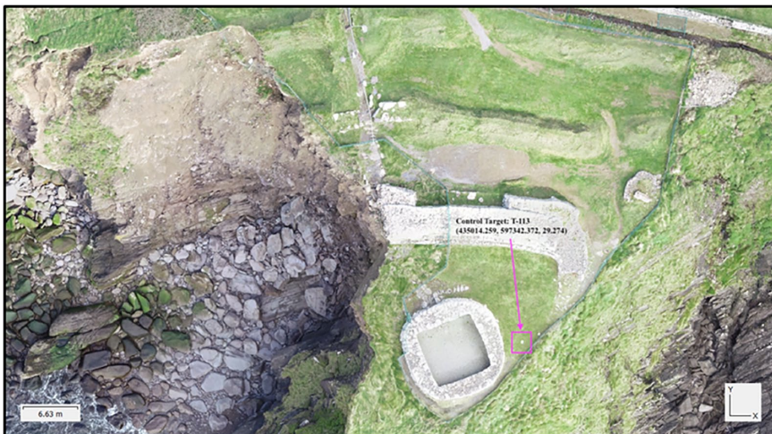
Figure 5. An orthogonal image from Dunbeg Fort. Adjacent to the stone feature is control target T-113 with its respective northings and eastings. Photo by Robert Shaw, Discovery Programme.
