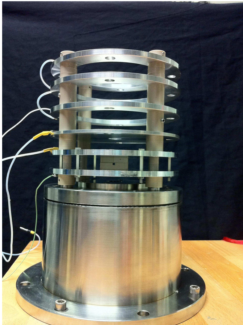
Figure 4.9: Photograph of the full ion optics stack with PEEK spacer. The path that the laser beam takes through the centre of the trap is clearly visible.
