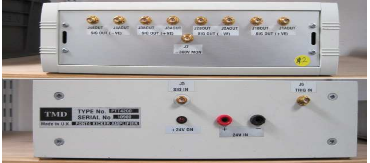
Figure 5.6: Photographs of the TMD kicker amplifier.
