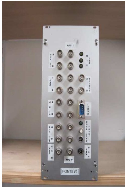
Figure 5.4: A photograph of the FONT5 board in its metal casing.
