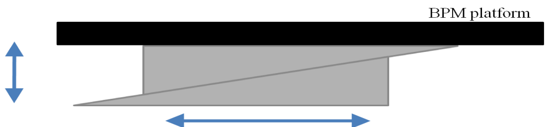
Figure 4.3: Diagram of the horizontal and vertical movers.
