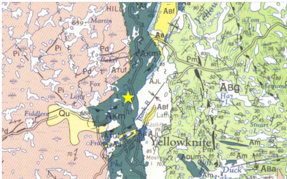
Figure 5-4: Zoomed in section of bedrock geology map by Henderson (1985) showing the pillow basalts symbolised as upside-down bowler hats in the dark green band. Yellow star marks the Giant Mine site
