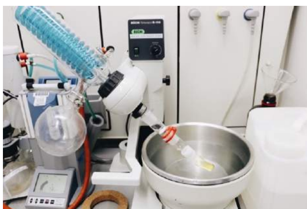
Figure 14: Extract being finalized in evaporator after transfer from round bottom flask
