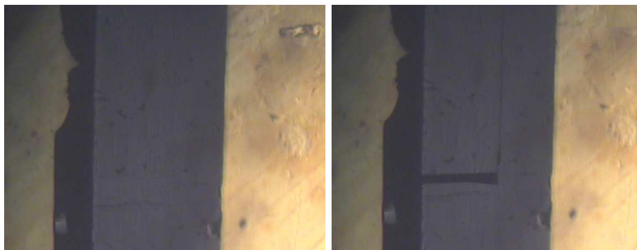
Figure 6.3: Mechanical twinning seen in TMTSF-PF 6 . Before (left) and after (right) force was applied to rear of sample
