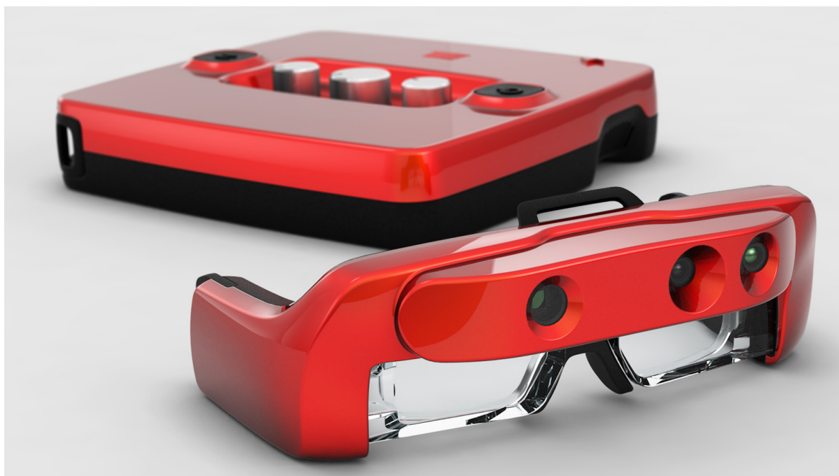
Figure 1-8 - Smart Specs. Control processing unit and headset. The control unit houses the image processor, battery and control electronics. The headset is comprised of an Epson BT-200 display, colour and depth cameras.
