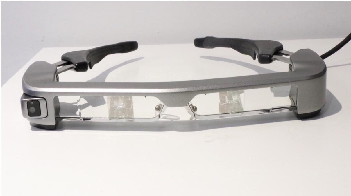
Figure A2- 1 BT35E Headset. The headset is identical to the Epson BT350; the difference is the display interface. The BT350 has a small handset containing a mobile processing unit, and the BT35E has an HDMI connection for interfacing with a separate computer.
