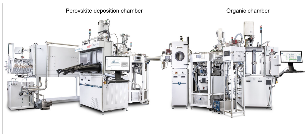
FIGURE 3.1: Photo of the national thin-film cluster facility. Only part of the facility (perovskite deposition chamber and organic chamber) is shown in the photo. Image credit: Angstrom Engineering.
