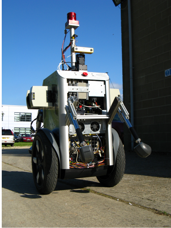
Figure 2.1: Data capture vehicle. A two wheeled dynamically balancing robot built around a RMP200 drive unit from Segway. Within the Dural mainframe there is an independent sensor payload consisting of battery packs, four networked PCs, a remote operation module and interface and power conditioning hardware for the vehicle’s sensor suite mounted on the vehicle’s periphery (see Appendix A for further details).
