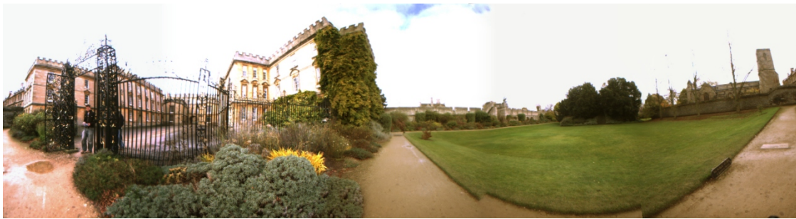
Figure 2.9: Typical panoramic image stitched together from the 5 cameras of the omnidirectional camera, mounted atop our research platform. To simplify the back projection of laser measurements we use only the single image that aligns closest with the field of view of the lasers (this also avoids unnecessary distortion of the images and visual artifacts such as those present along the grass verge in the image). The person in the image is standing at the interface between the “Campus” environment (the other side of the large wrought iron railings) and the “Parkland” environments. This entrance gate was only marginally wider than the research platform which led to a prolonged navigation surrounding this area. As discussed in Section 2.4.5 and shown in Figure 2.14, this navigation resulted in an accelerated accumulated error in trajectory estimation for this region.
