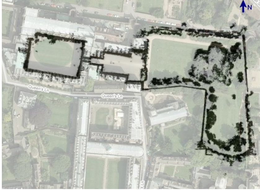
Figure 2.14: Ariel view of the New College test site with laser measurements superimposed. The point cloud was manually stretched and rotated to fit the aerial view based on the vertical structures that appear in both representations of the workspace. We see that overall there is a high level of agreement between representations, bar a rotational error in trajectory estimation surrounding the interface between “Campus” and “Parkland” environments near the centre of the figure. This led to an angular error of the “Parkland” point cloud relative to the overhead image.
