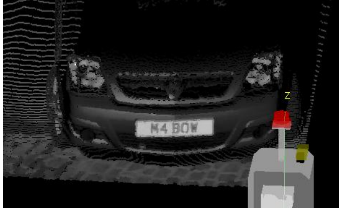
Figure 2.8: Small section of laser data that embodies the front of a car. Data was generated using the tools detailed in Section 2.3.1. Colouring of points is supplied by laser reflectance. One can clearly discriminate coherent letters on the car number plate which are as a result from black lettering on a reflective backing.
