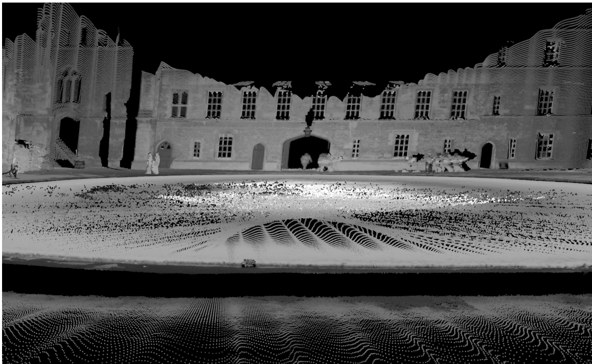
Figure 1.1: Laser point cloud of the New College quadrangle, Oxford, using data collected from our robotics research platform. As humans we can easily parse the workspace surfaces that are present in the laser data, but can a more efficient representation be created that can permit direct and automatic access to these underlying surfaces?
