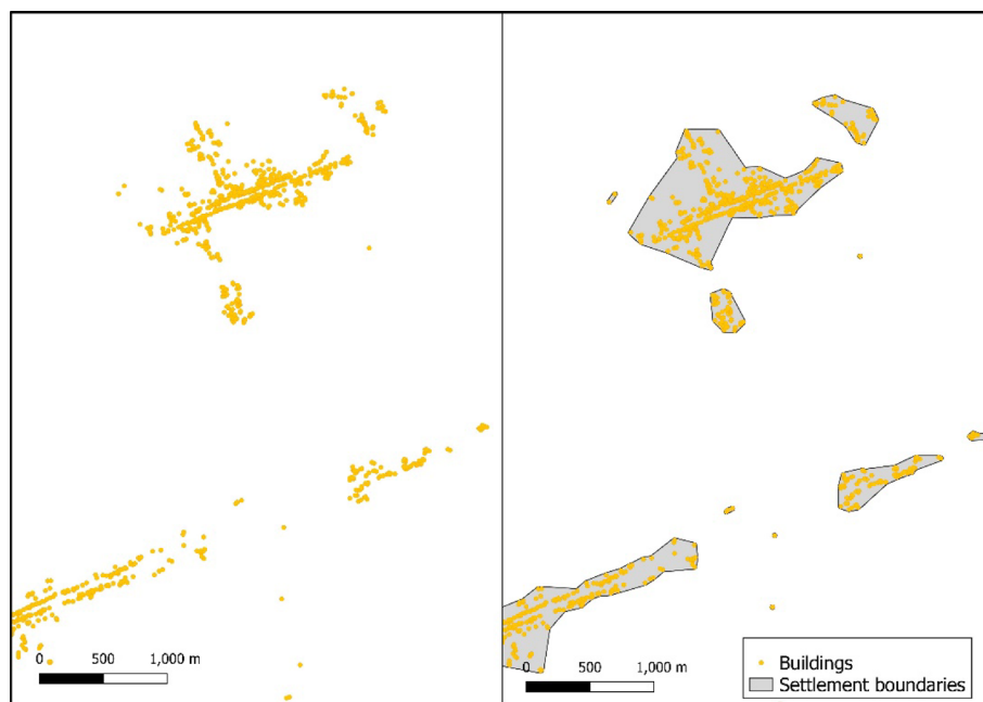
Fig. 3 Updated clustering algorithm based on building data. On the left are the individual building footprints, and on the right are the clustered buildings and the alpha shape cluster geometries
