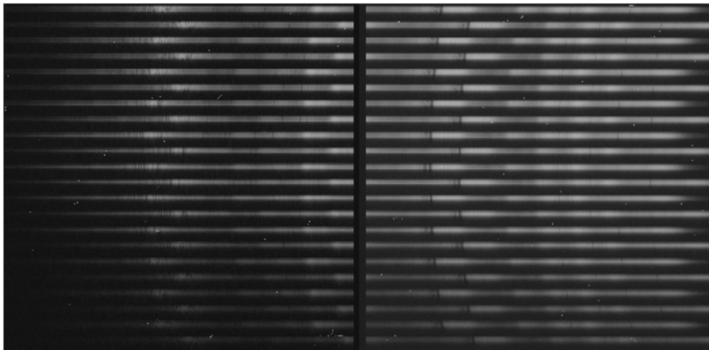
Figure 2.4: A sample of a raw, uncalibrated Palomar SWIFT image of Neptune. This is the ‘master’ image, produced by breaking the lower half of the original field of view into one long slit, and then breaking this slit into the 22 slitlets which appear here as horizontal lines. Each of these lines contains spectral information in the horizontal direction and 7.12” of spatial information (at 0.08” resolution) in the vertical direction.
