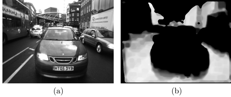
Figure 5.12: Example distraction suppression mask generated online using stereo and a 3D pointcloud Scene Prior. Taken from [64], courtesy of Colin McManus. On the left, an image from dense traffic in central London, on the right a distraction suppression mask generated online using dense stereo compared against a 3D pointcloud Scene Prior captured earlier. The image is coloured according to the confidence of the prior being visible, with white denoting high confidence and black denoting low confidence. Thus areas coloured black are believed to contain distractions, rather than the prior and should not be used for localisation, as they contain dynamic objects.
