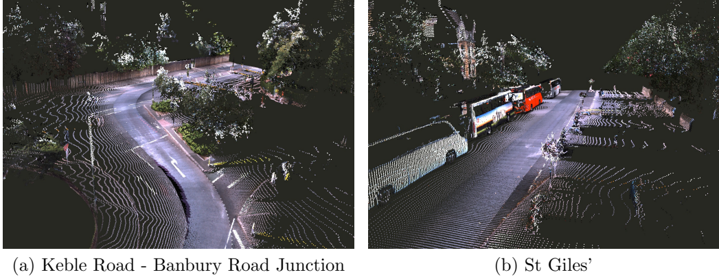
Figure 8.33: Examples of areas where the Scene Prior provides poor structural confinement, taken from dataset B1. Both of the areas shown are areas in which LAPS frequently fails to produce positively classified poses and thus trigger LAPS restarts. The common theme is that there are no buildings sampled in the prior, and thus the only structure above the ground plane are trees which often have a homogeneous appearance. This absence of strong appearance cues for alignment on the structure results in either poor confinement, or no clear minima in the NID. In some cases, as in Figure 8.33b, this problem is partly a function of traffic. In the case shown, the buses are blocking the view of structure which would otherwise be useful for localisation.
