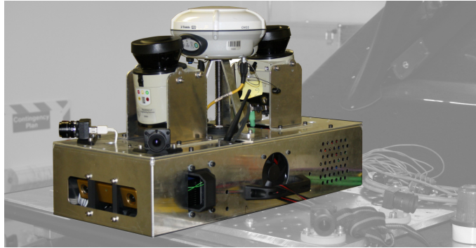
Figure 3.28: NABU: Mounted on the Wildcat. The NABU mounted on the MRG Wildcat. Visible are the PointGrey FireFly cameras (front-left, front-right), the SICK LIDARs (both inclined and declined) and the Trimble R8 GPS unit.
