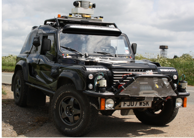
Figure 4.1: The MRG “Wildcat” . The Wildcat is a heavily-instrumented platform initially developed by BAE systems. The vehicle is equipped with an Oxford Technical Solutions INS and a host of sensing modalities including LIDAR and camera units.
