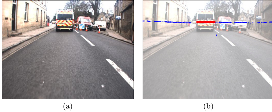
Figure 6.14: Woodstock town centre. (a) An example LIDAR sweep at the \lambda_{TC} position as viewed from an onboard camera, and (b) with the horizontal LIDAR points overlaid. This fan corresponds to the scene shown in Figure 6.9. The points falling on the vehicle in front (highlighted in red) must be filtered out to prevent the velocity error highlighted in Figure 6.9.
