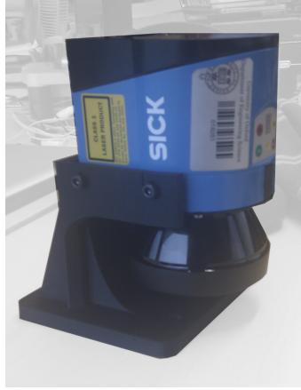
Figure 2.7: SICK scanning LIDAR. A SICK LMS-151 scanning-LIDAR unit, used throughout this thesis. The unit in this image is mounted upside-down in a custom, rapid-prototyped mount.
