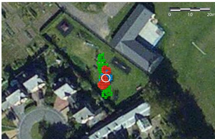
Figure 11: Raw positions of 3 GPS units in three different orientations, rotated on a roundabout. Colours correspond to angle of the units; red = 0°, blue - 45° and green = 90°. The white circle shows the approximate circumference of the roundabout (1.5m radius). It is evident that when the GPS is oriented at 90°, the signal is less accurate.
