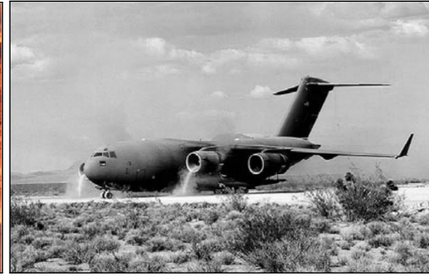
Figure 2: Sand ingestion by a C-17 at takeoff (Walsh et al., 2006).
