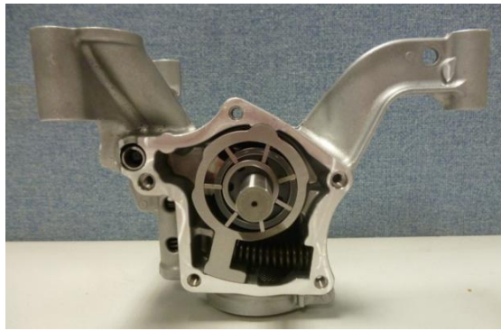
Figure 54. SHW VDOP oil pump fitted to the 1.0 Ford EcoBoost engine. The image shows the pump with the front cover removed.
