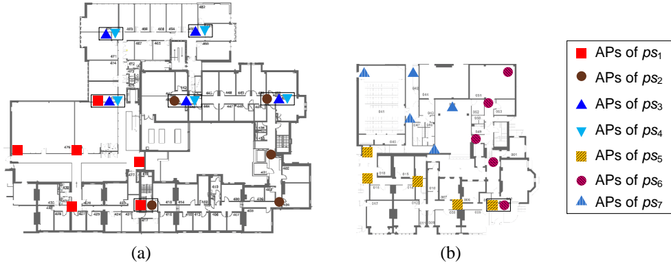
Figure 6.7: (a) The WiFi access points deployed for 4 different WiFi+IMU positioning systems ps_1 , ps_2 , ps_3 and ps_4 on the 4th floor testbed. APs shared by different systems are marked with the rectangles. (b) The WiFi access points deployed for 3 different WiFi+IMU positioning systems ps_5 , ps_6 and ps_7 on the basement testbed. APs shared by different systems are marked with the rectangles.
