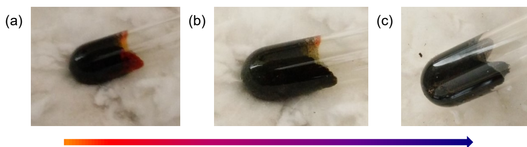
Figure 7-5. Photographs of the ampoule (a) when removed from the furnace at 500 °C, (b) while cooling, and (c) when rapidly cooled to room temperature.
