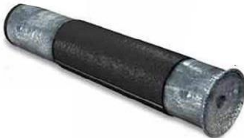
Figure 3.1: The original three-lens microscope produced by Zacharias and Hans Janssen, now on display in Middleburg, Netherlands[109].
