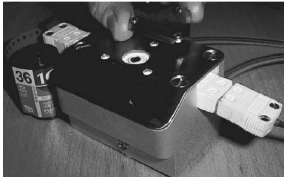
Figure 3.12: Philips Electroscan ESEM hot stage with shielding lifted to reveal resistive heating element [158].
