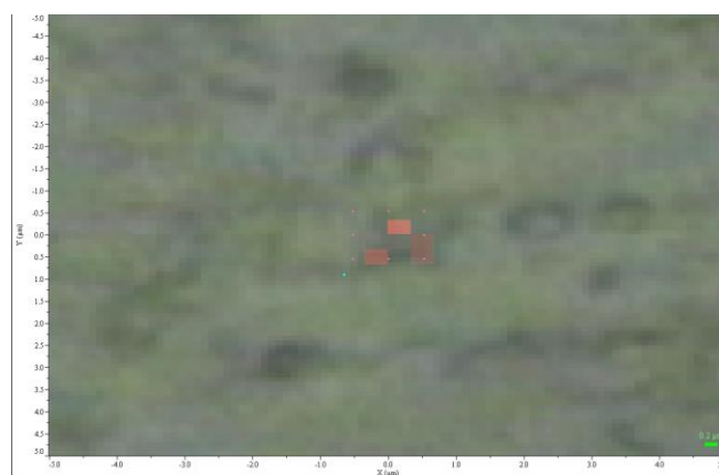
Figure 5.6: Spatial distribution of Raman signal from 2000 to 2200\text{ cm}^{-1} in a 3\times 3 pixel map of E. coli
