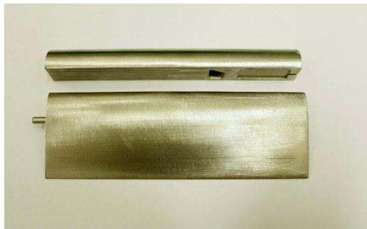
(a) View of suction surface of blade.
