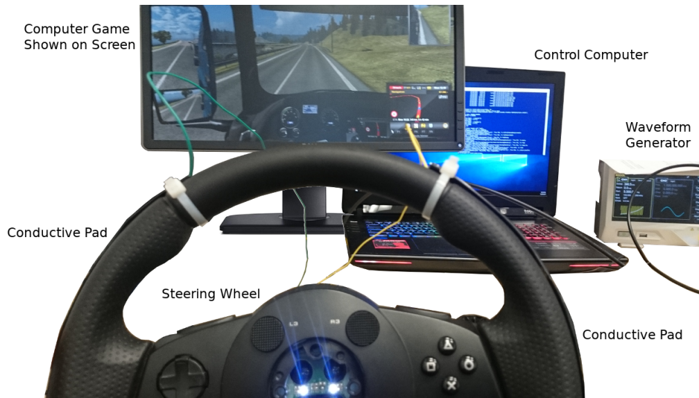
Figure 5.8: Experimental set-up from the perspective of the test subjects. The steering wheel controls the vehicle in the computer game shown on the screen in front of the participants.
